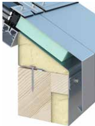
Installation on wood upstand
